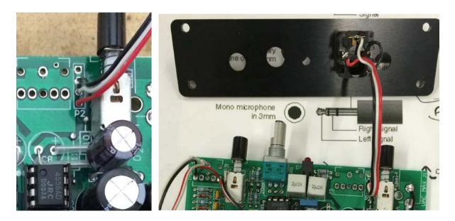
Attach headphone jack to front plate after completing all other assembly. Black nut is secured by a compression fit. With jack & nut installed on front plate, use table surface to apply pressure to nut. After nut snaps in place, gently rotate 1/4 turn clockwise.
