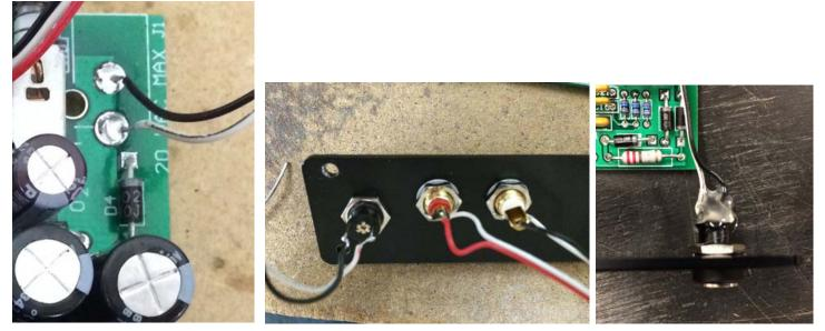
2) Apply hot glue to connectors as shown. Let glue dry before installing into case.
