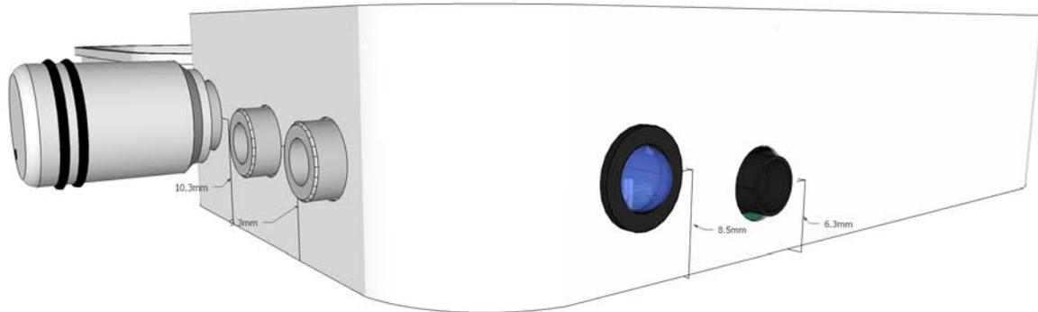
2. Punch holes at the marked locations with a hole punch. Vertical heights are not critical, but are provided for reference in the image at right. Ensure the holes will not interfere with the lid (remember to account for the audio jack nuts). Holes for the audio jacks, the LED, and the DC jack should require a single punched hole. The volume potentiometer hole will need to be enlarged by punching multiple holes. This unsightly hole will be hidden by the volume knob.
