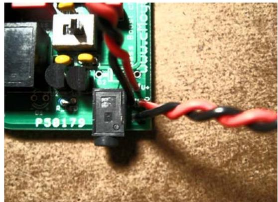
Increasing the supply voltage to 18V enables higher volumes when driving high impedance headphones (typically 64 ohms and above). Two batteries in series will drain somewhat faster than a single battery. This modification also adds weight to the amplifier and adds slight difficulty when changing batteries due to the very tight fit. Most people with 120 ohm headphones and less are pleased with a single 9V battery, therefore, we only recommend using 18V if you find 9V to be insufficient.
