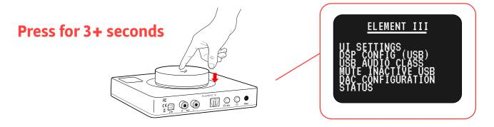
Pressing down on the Volume Knob for 3+ seconds enters the Options Menu (shown below). Turn the knob to navigate up/down the options menu. Push the knob to make a selection.
