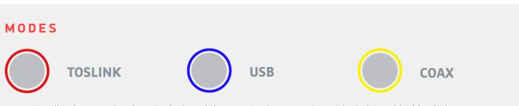
Your PC will only recognize the USB device while EL DAC II is set to USB mode, indicated by blue light.
